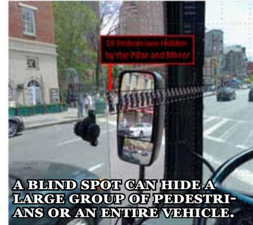
fixed by narrowing the A pillars and moving and reducing the size of the left side mirrors so drivers can readily see approaching pedestrians and vehicles from all angles without moving like a boxer in a fight. The correction can cost as little as \$300 per bus.
